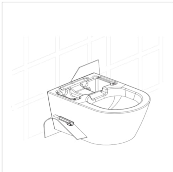
19. Using a Stanley Knife, remove any exposed 'Damper Cushion' that protrudes from behind the Toilet's Structure.
